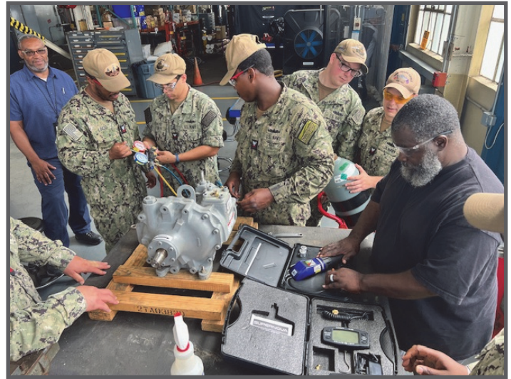
MM2 Gilkey and MM1 Lindo pressure testing on a reciprocating compressor. (Photo by Cedric Ridley.)
