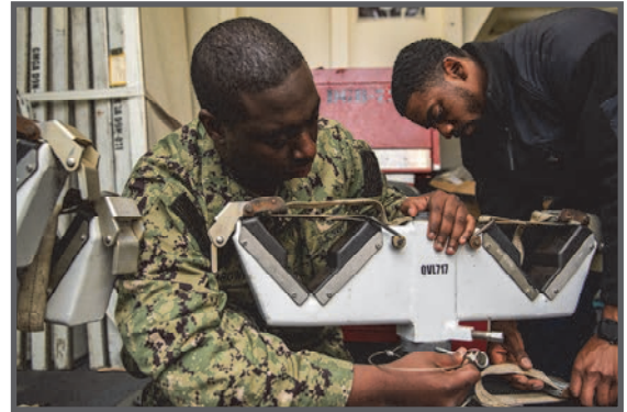
SAN DIEGO – Aviation Ordnanceman 2nd Class Shaquille Brown, a native of West Palm Beach, Florida, and Aviation Ordnanceman 3rd Class Demonta Martin, a native of Montgomery, Alabama, inspect an adjustable weapons adapter ADU-514 in the Armament Weapons Support Equipment storeroom aboard USS Boxer (LHD 4). Boxer is a Wasp-class amphibious assault ship homeported in San Diego. (U.S. Navy photo by Mass Communication Specialist 2nd Class Roland Ardon)
