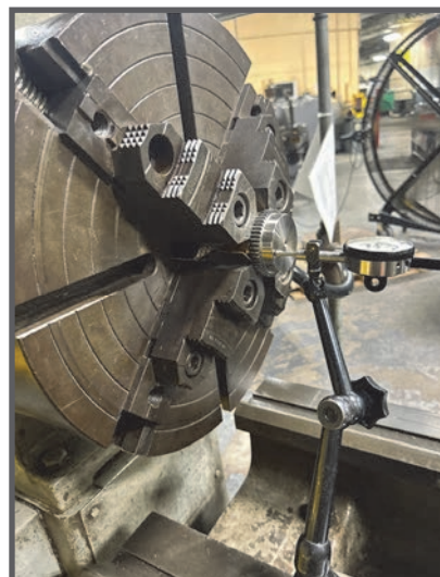
The pump coupling as it was being prepared for internal boring on a lathe by MR2 (SW) Kayla Smith at Mid-Atlantic Regional Maintenance Center. (Photo by MR2 (SW) Andrew Everoski.)
