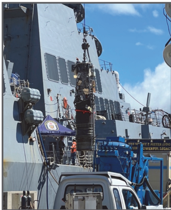
Gas Turbine Generator (GTG) is being rigged out of USS Wayne E. Meyer for swap out. (Photo by GSM1 Joseph Pennington.)
