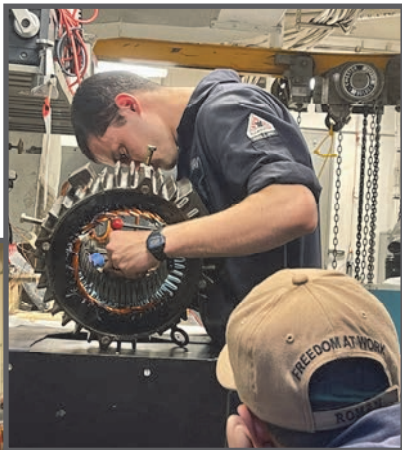
Above: Work Center Supervisor, EM2 Josh Roman, supervises as EM2 John Walsh lays alpha phase coils in a 440v three-phase electrical motor. (Photo by EM3 Kevin Vicentesolis.)
