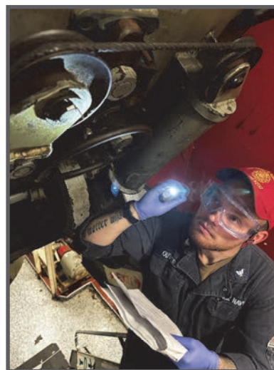
DC3 Wyatt Oliverson inspecting hatch for loose, missing, and/or damaged parts, or parts showing excessive wear or corrosion. (Photo by MRCS (SW/AW) Brian Pierce.)
