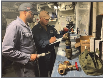
USS Harpers Ferry (LSD 49) Auxiliary Division Sailors MM3 Alberto Sanchez (left) and MM1 (SW) Ronald Dumale, who are enrolled in the NAMTS Valve Repair Technician JQR, receive general valve maintenance mentorship on a relief valve and a globe valve. (Photo by Steven Constantino.)
