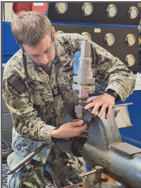
MM1(SS) Joshua Ogletree prepares to pop test a high pressure relief valve from the USS New York (LPD 21). The relief valve is an important part of the ship's Reverse Osmosis water system that provides potable water to the crew. (Photo by Reginald Kitchens.)
