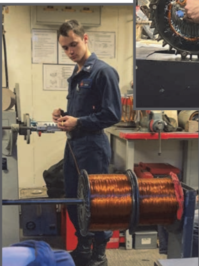
Above: Work Center Supervisor, EM2 Josh Roman, supervises as EM2 John Walsh lays alpha phase coils in a 440v three-phase electrical motor. (Photo by EM3 Kevin Vicentesolis.)
