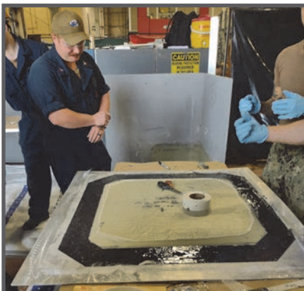
Stop sign patch with the Polysulfide sealer applied. (Photo by Andy “Rusty” Vasquez.)
