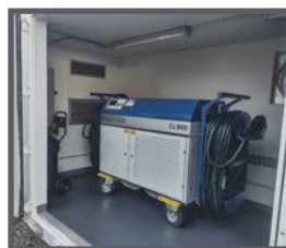
CL 1000, a high-powered cleaning laser provided by Adapt Laser Systems, LLC, who provided units in Norfolk and San Diego.
