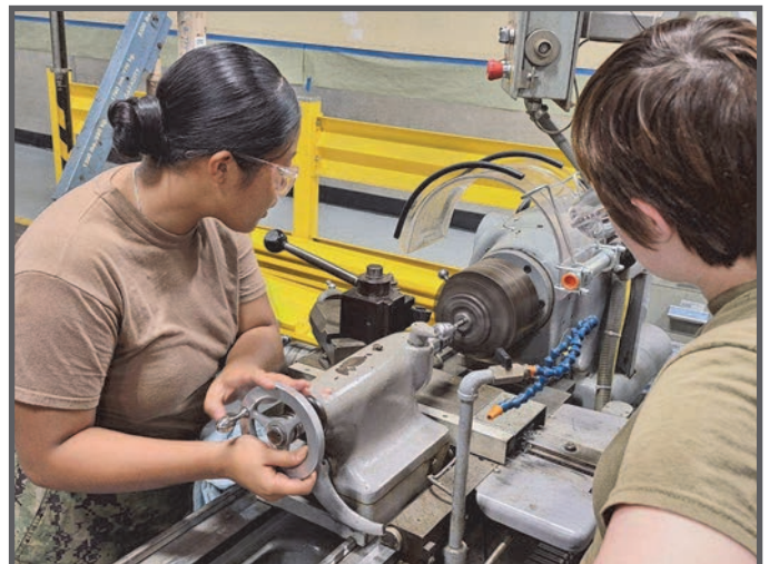
MR3 Mariloumae Manantan (left) and MR2(SW) Hannah Swearingen (right) use a Monarch EE Lathe to manufacture a threaded component for a NIXIE transom handle on USS Mitscher (DDG 57). (Photo by Reginald Kitchens.)
