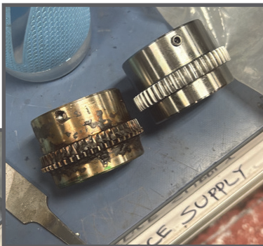
The damaged & new Anchor Windlass pump coupling aboard USS Carney (DDG 64). (Photos by MR2 (SW) Andrew Everoski.)
