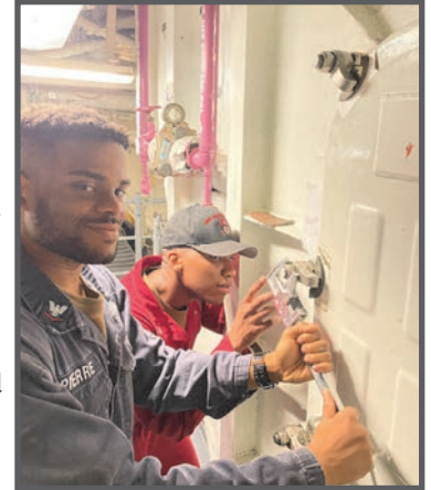
Left to right are NAMTS Afloat Watertight Closure Maintenance Technician NEC graduates DC3 (AW) Wadnelito Andre and DC3 (SW) Pierre LaPierre from USS Makin Island (LHD 8) adjusting a QAWTD using Method One.
