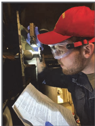
DC3 Wyatt Oliverson is performing maintenance on a watertight hatch. The maintenance consists of test, clean, inspect and lubricate hatch/door. (Photo by MRCS (SW/AW) Brian Pierce.)
