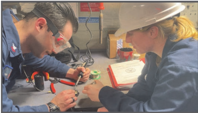
EM2 John Walsh and EM3 Riley Quinn apply solder to an overload relay. (Photo by EM3 Kevin Vicentesolis.)
