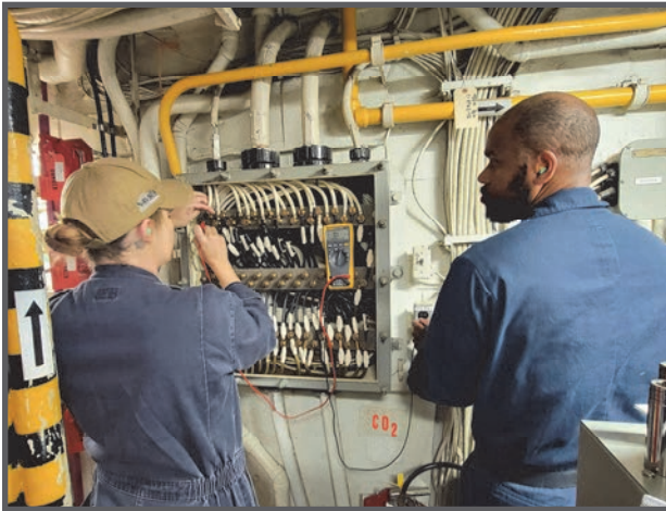
EM1 Nicole Yorgesen and EM2 Patrick Jones from Southwest Regional Maintenance Center work to isolate a ground on the ship's degaussing system. (Photo by Russ Lincoln.)
