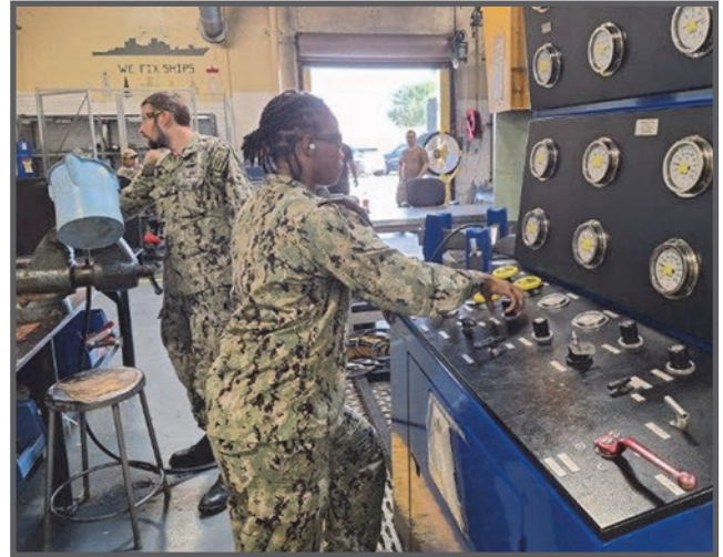
MMFN Jalayssia Washington operates MAMCs hydrostatic test stands that provides the necessary pressure to test relief valves. A high pressure relief valve from the USS New York (LPD 21) is pictured here being tested to 1,050psi prior to being sent back the ship for install. (Photo by Reginald Kitchens.)
