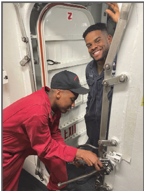
Left to right are NAMTS Afloat Watertight Closure NEC graduates DC3(AW) Wadnelito Andre and DC3 (SW) Pierre LaPierre of the USS Makin Island (LHD 8) adjusting a QAWTD Operating Handle.
