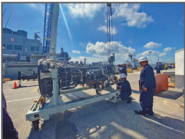
Last minute Quality Assurance checks on the new 2A GTM before being lifted onto USS Carney (DDG 64).
