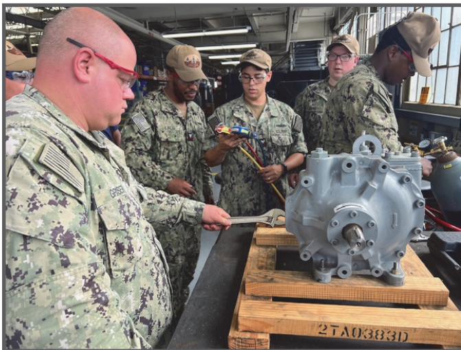
MM2 Dubose demonstrating a pressure test and leak testing on a reciprocating compressor. (Photo by Cedric Ridley.)
