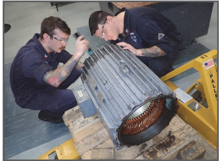
EM1 (SW) Ryan Nelson and EM1 (SW) Declan Faulkner doing an internal motor inspection. (Photo by MM2 (SW) John Rabanes.)
