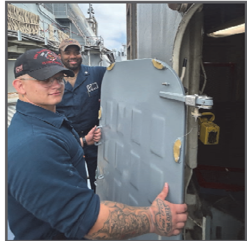
USS Harpers Ferry's (LSD 49) DCFN Joshua Neu and OS3 Del Dennis, who are assigned to the ER09 Damage Control Petty Officer Work Center, prepare to install a watertight door on August 02, 2023. This newly refurbished door will have its hinge assembly upgraded. (Photo by Ramir Púlido, NAMTS Mentor.)
