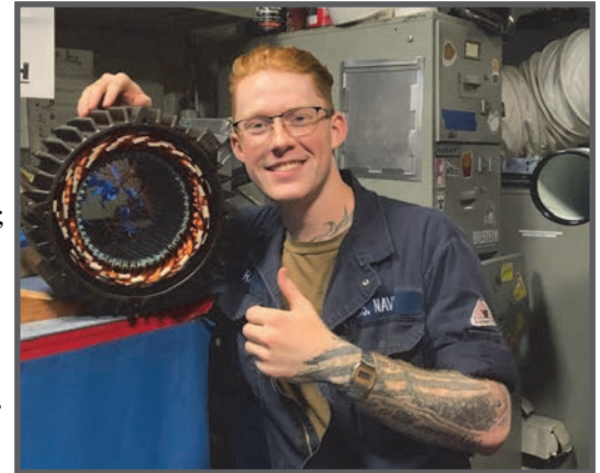
"There were two mission critical motors, one for a lube oil pump and one exhaust motor that were sent to us from a destroyer that I was involved with rewinding. There was another motor from a cruiser that was also sent to us that we repaired for them," said EM2 Joshua Riggs. (Photo by EM2 Walsh.)
