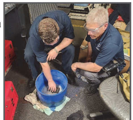
FN Kyle Bengford smooths the surface of the underside of the valve test stand table using a precision block and 900 grit crocus cloth. Outside Machine SME Mike Dengate waits for FN Bengford to clean the surface so it can be checked. (Photo by Jon Bonet.)
