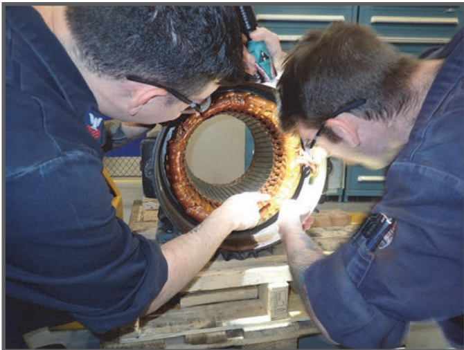
EM1 (SW) Ryan Nelson and EM1 (SW) Declan Faulkner inspection of the bake light/varnish of the motor. (Photo by MM2 (SW) John Rabanes.)
